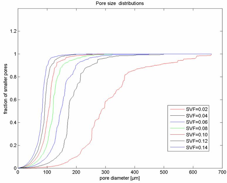
**Figure 5:** Pore size distributions for various SVFs, Experiment A.
