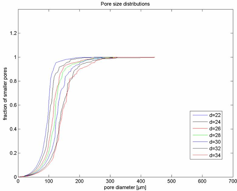
**Figure 6:** Pore size distributions for various fiber diameters, Experiment B.
