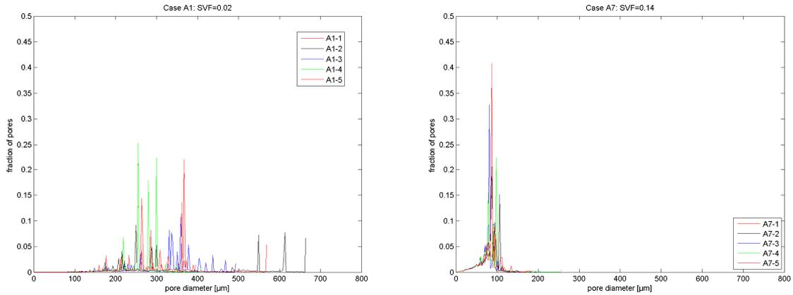
**Figure 4:** Pore sizes distributions for five realizations of SVF 0.02 (left) and for five realizations of SVF 0.14 (right), Experiment A. The variation is much higher for smaller SVF.
