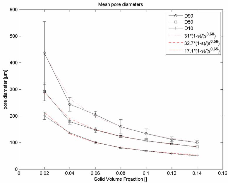
**Figure 7.** Variation of D10, D50 and D90 depending on grammage.
