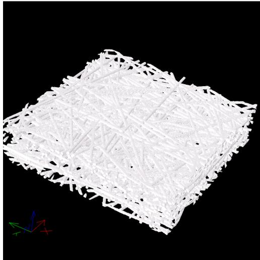
**Figure 1:** 3d visualization of a generated nonwoven (from [10], using [13]).
