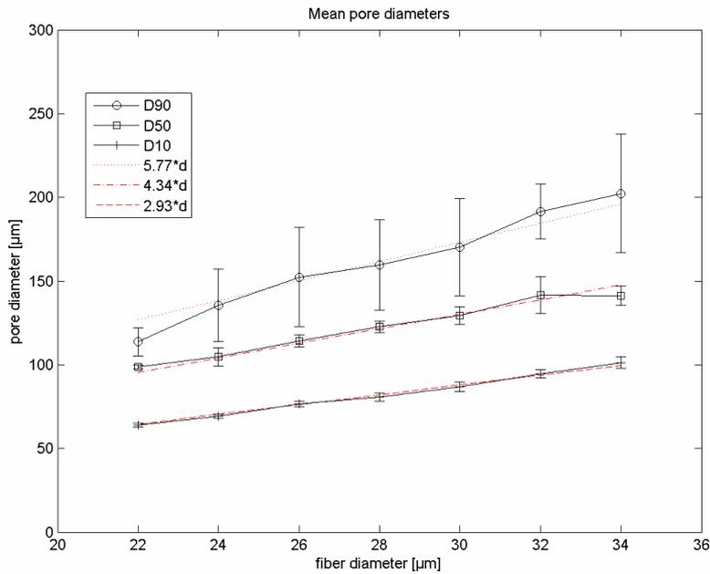
**Figure 8.** Variation of D10, D50 and D90 depending on fiber diameter.
