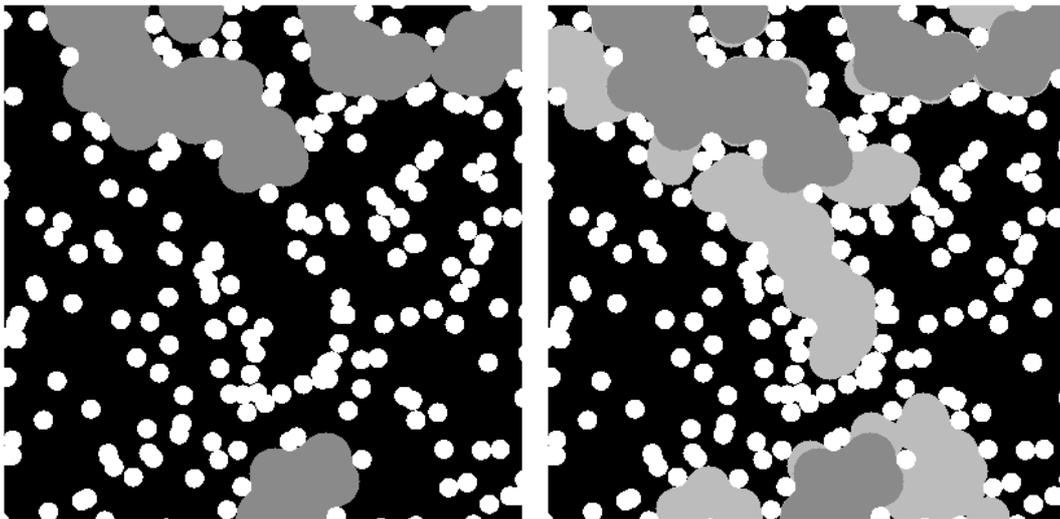
**Figure 2:** Two dimensional view illustrating the method of a mercury intrusion porosimetry simulation. Fibers are white, and grey areas indicate pores of radius  $r \geq 20$  and  $r \geq 16$ , respectively. All marked pores are always connected to one of the mercury reservoirs on top or bottom of the sample by a wide enough path. (from [10], using [13]).
