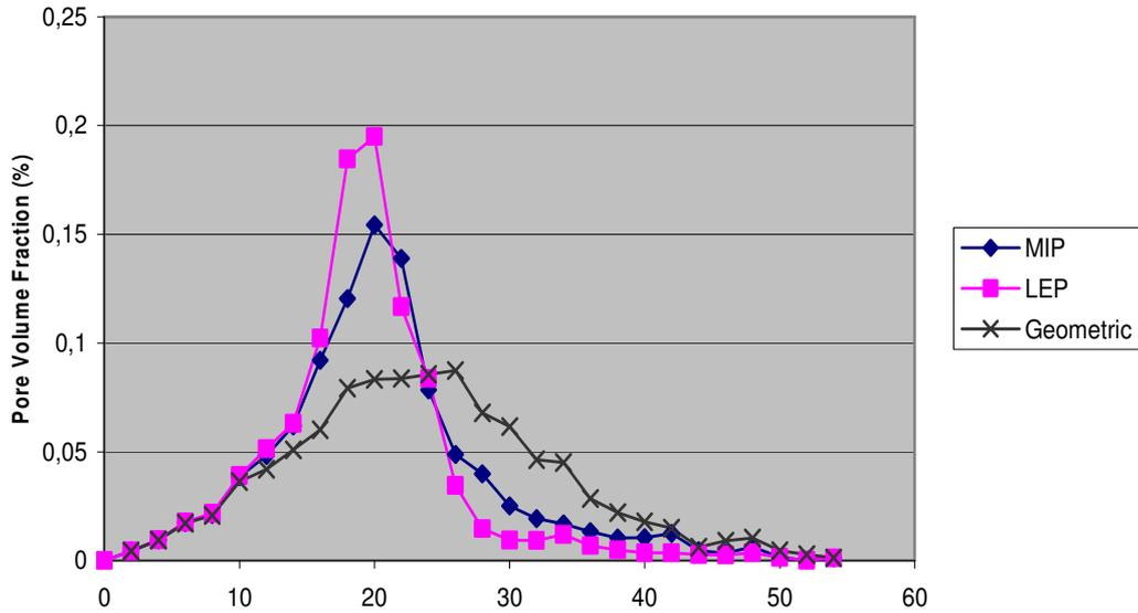
**Figure 3:** Pore size distribution of the sample shown in Figure 1. The diagram shows the calculated geometric pore size distribution and the results of the simulated mercury intrusion porosimetry (MIP) and the simulated liquid extrusion porosimetry (LEP) (from [10]).
