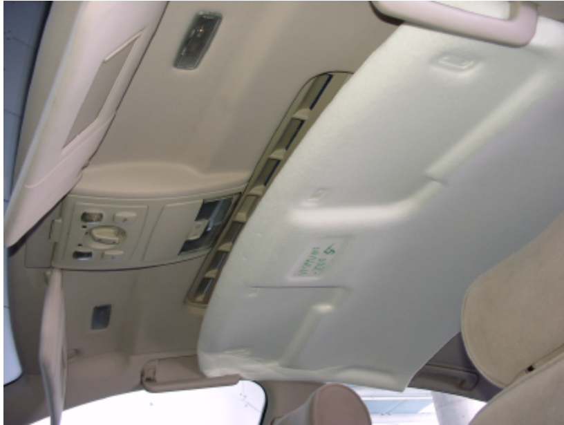
Acoustic trim for the interior of the car: Headliner made of fleece
