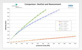
velocity dependent pressure drop for perfusion with air, comparison between experiment and simulation:
