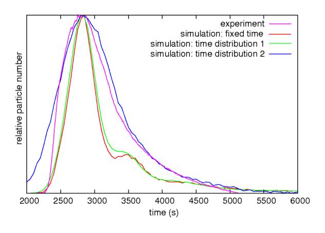
experiment: 66.8 µL/min, exact times and positions of particles entering the fracture unknown
