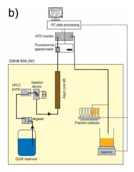
the nanoparticle (quantum dots) transport is experimentally realized by means of column migration experiments at the KIT, Institute for Nuclear Waste Disposal
