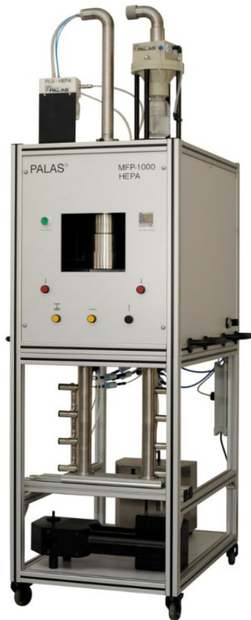
Single-pass filtration test rig MFP 1000 from Palas GmbH
