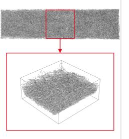
The AI separates the solid voxels in the image data into individual fibers.
