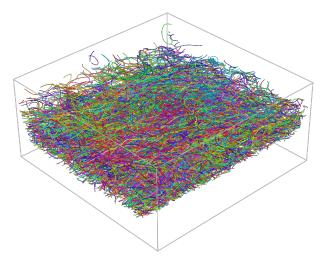
Geometric information, such as fiber length, fiber segment orientation & fiber diameter, can be read directly from the object.
