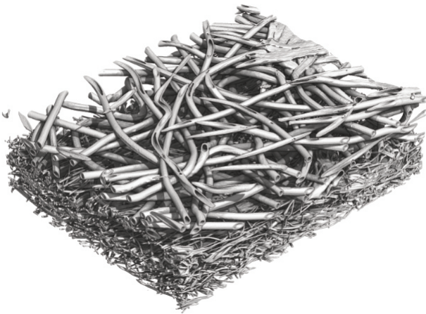
Result: Digital model of the filter media and its statistical description
