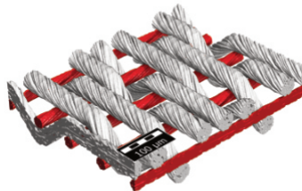
Multifilament reverse Dutch weave
