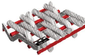
Multifilament reverse Dutch weave
