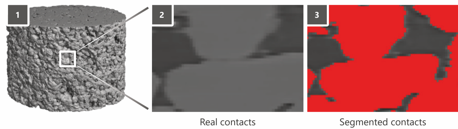
Illustration of a common limitation in standard DRP workflows: 1: 3D visualization of Gildehauser sandstone [4] 2: 2D μCT slice showing pore space and mineral grains 3: Grain-contact features unresolved during segmentation due to limited scan resolution.
