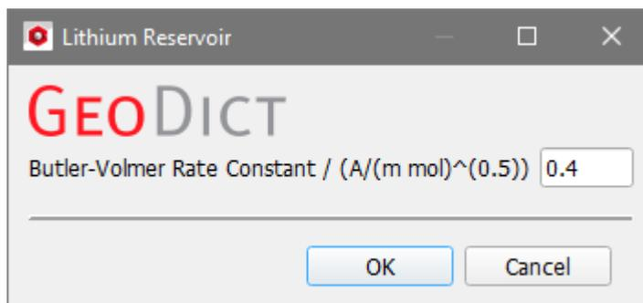
No other parameters need to be set for a lithium reservoir, since it will be considered as a never-ending reservoir of lithium, not limiting the battery performance.
