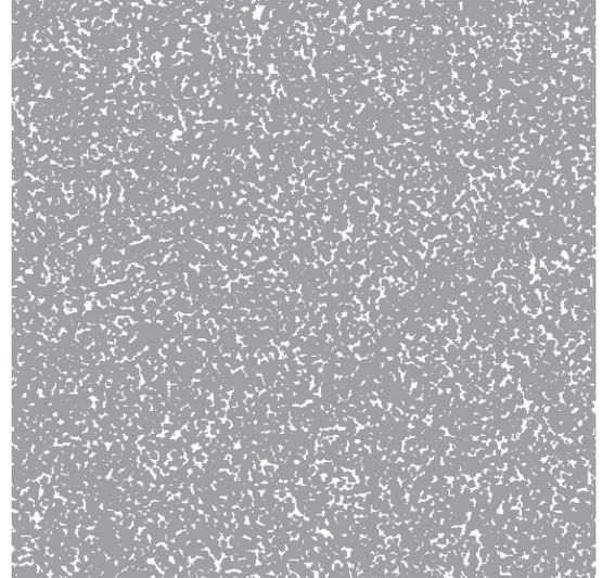
The electrical conductivity of the structure, for pores filled with brine, is computed with the EJ and the LIR solver. For sandstone, an electrical conductivity of 1e-08 S/m and for the brine of 5 S/m is used as input values.
