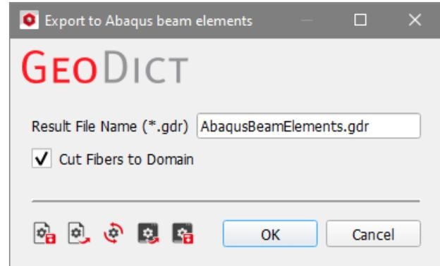
In the **Export to Abaqus Beam Elements** dialog, choose a **Result File Name (\*.gdr)** according to the current project. The result file contains all information about the current export. The corresponding result folder contains the input files for Abaqus and the chosen structure.
