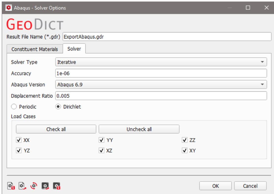
Select the **Solver Type** for the simulation in Abaqus with the corresponding dropdown menu. The available options are **Direct** or **Iterative**.
