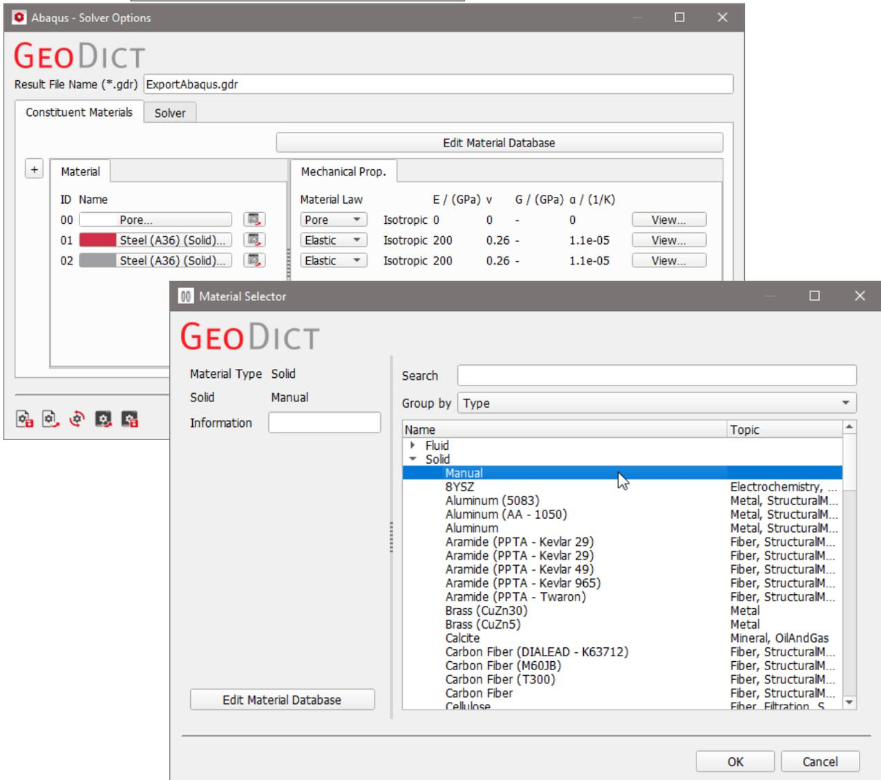
Under the **Constituent Materials** tab, set the constituent materials for Material ID 00, Material ID 01, and Material ID 02 to **Solid** → **Manual** through the Material Selector.
