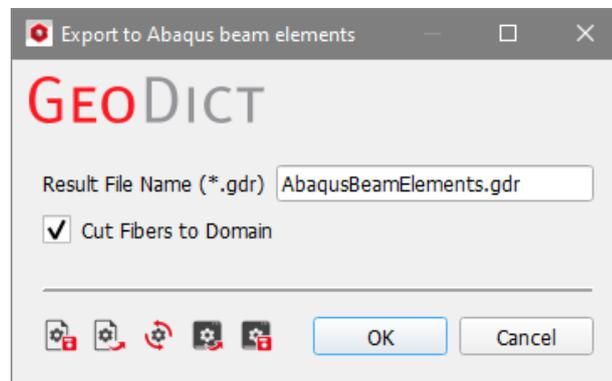
In GeoDict, fiber objects can be larger than the domain. This has no effect on GeoDict simulations, since all GeoDict simulations are limited to the domain. However, fibers which leave the domain may lead to unexpected results in other simulation software, such as Abaqus. Therefore, it is recommended to keep **Cut Fibers to Domain** enabled.
