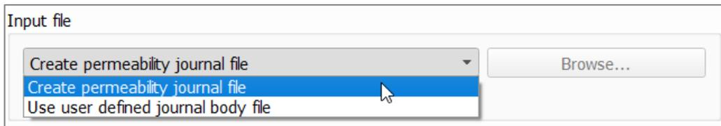
The **Fluent™** manuals explain how to create **Fluent™** journal body files (\*.jbf). Several journal body files (**pressureDrop\_X.jbf**, **pressureDrop\_Y.jbf**, **pressureDrop\_Z.jbf**, and **massFlux.jbf**) are included as examples in the **ExportGeoFluent** folder in the **GeoDict** installation directory (e.g. C:\Program Files\Math2Market GmbH\GeoDict2022\ExportGeoFluent).
