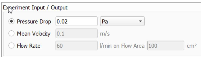
For a given **Pressure Drop** as experiment input, the output is the **Mean Velocity** and vice versa. The **Pressure Drop** is the difference between the inflow and outflow pressures, and the **Mean Velocity** is the average speed of the flow in the flow-direction.
