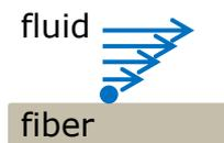
A non-zero **Slip Length** simulates the sliding of the fluid along the structure' fibers, increasing the fluid mean flux and thus, the permeability of the filter. This option might be used when it is realistic for a given physical material. Currently, the same slip length value must be set for all materials in the structure.
