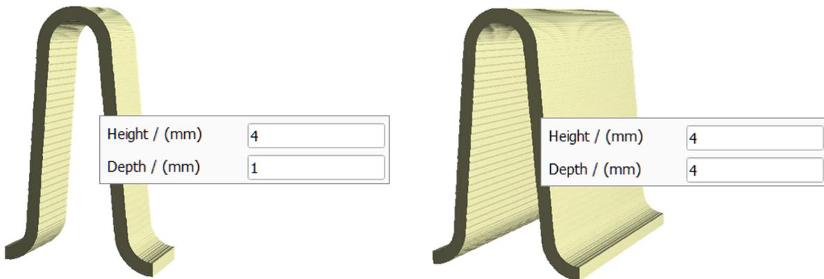
The values of **Radius at Pleat Tip** and **Radius at Pleat Valley** determine the upper pleat radius and lower pleat radius measured at the upper or the lower folds of the pleat.
