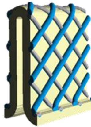
The netting or weave **Tilt Angle** is the angle of incline of the netting or the weave supporting structure with respect to the pleat medium along the pleat depth. The valid tilt angle values range from 0° to 45°.
